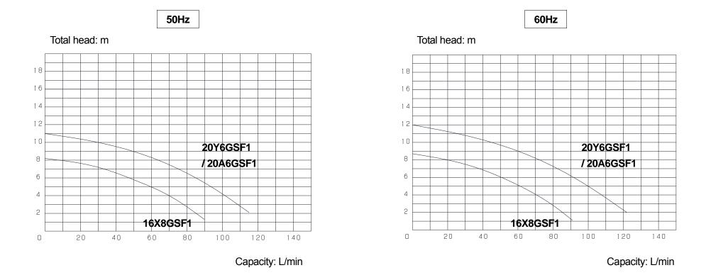
This performance test is based on JIS B 8301, 8302. The specific gravity of test liquid is 1.0.
