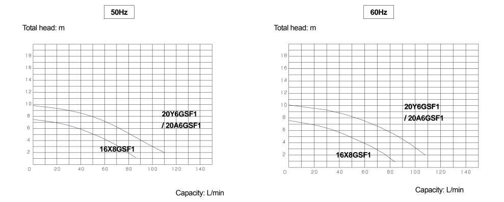
This performance test is based on JIS B 8301, 8302. The specific gravity of test liquid is 1.0.
