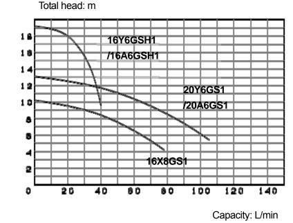
This performance test is based on JIS B 8301, 8302. The specific gravity of test liquid is 1.0.
