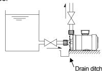
In this regard, if the liquid level from the suction inlet of the pump is too low, air enters, may cause pump failure. Make sure air not to enter. Become the height 30 mm as much as possible.
