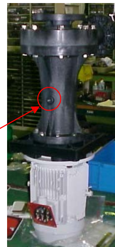
Air-release bolt with gasket
