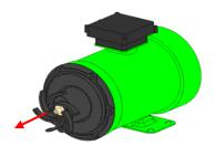
4 The rear casing can be removed forward by slightly lifting with sharps which are put into the matching face to the bracket.
