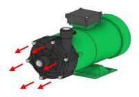
③ Pull out the impeller forward. Be careful not to damage the parts. In doing so, it gets back to afterward by the magnet force. Be careful not to catch your fingere
