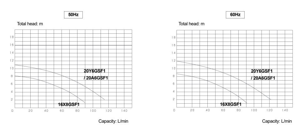
This performance test is based on JIS B 8301, 8302. The specific gravity of test liquid is 1.0.
