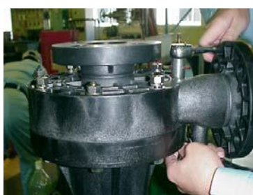
Tighten the rest of six bolt holes 1 bolt+ 2 washers+1 spring+1 nut
